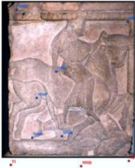
Figure 11. Orthophoto with control (red) and check (blue) points
