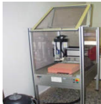
Figure 15. Numeric controlled milling machine ABAMill 4433
