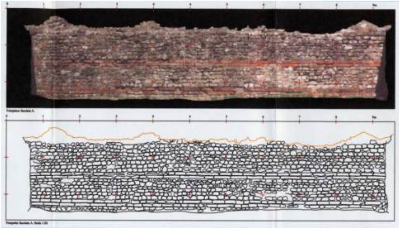
Figure 7. Digital rectification of a wall and its vectorial drawing
